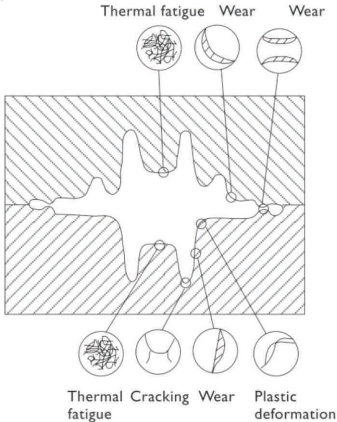
**Fig. 1: Overview of forging die failure mechanisms [1]**
