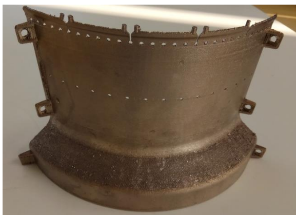
Figure 2. Manufactured combustion chamber segment.
