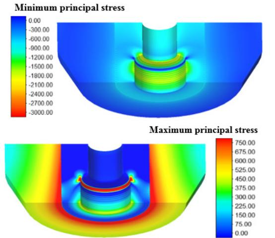
Fig. 5 Moving die; minimum and maximum principal stresses.
