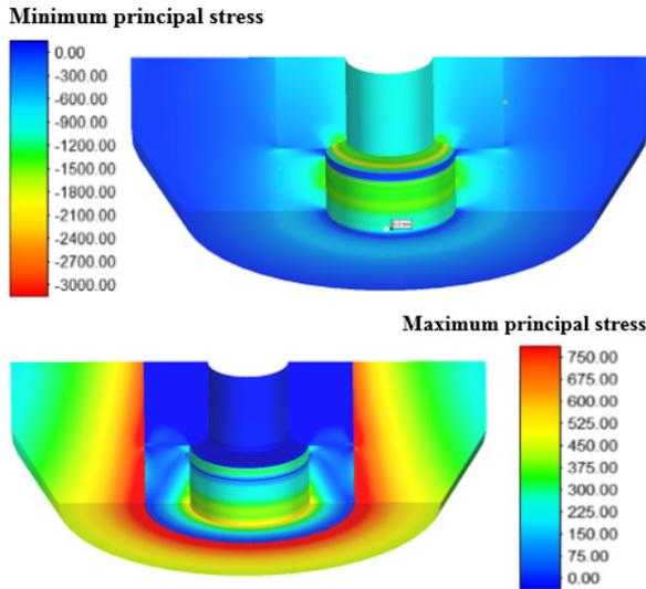
Fig. 7 Revised tool design; minimum and maximum principal stresses.
