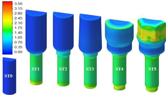
Fig. 3 Distribution of effective plastic strain on forging stages.
