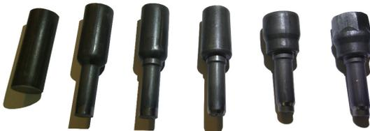
Fig. 9 Stage designs and final product obtained from the production.
