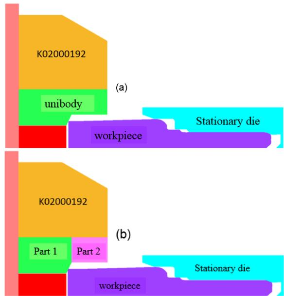
Fig. 6 Schematic representation of the moving design of fourth stage; (a) Current design, (b) Split design. Part 1 and Part 2 are the split moving dies.
