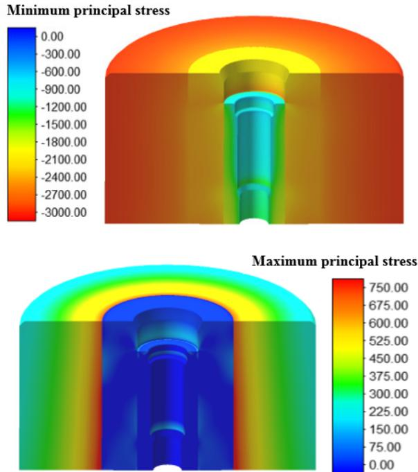
Fig. 8 Stationary die; minimum and maximum principal stresses.
