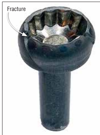
Figure 4. Fracture on cold-forged bolt
