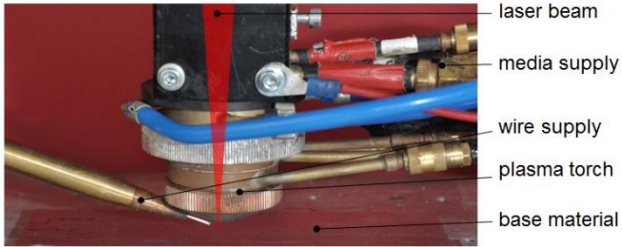
Fig. 1. Coaxial set-up for fluxless hybrid laser-plasma brazing (BIAS ID 160081).
