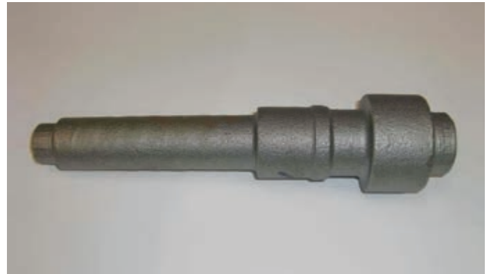
After Inductive Heating to 1240 Degrees, the Component Is Formed on a Cross Wedge Roll
