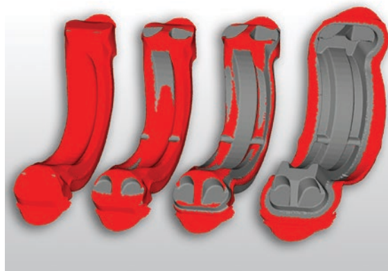
The simulated deformation during finisher using the corrected shape from blocker was formed without lap
