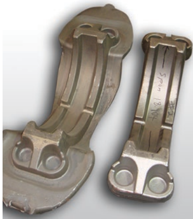
Blocker part with flash and the trimmed finish part
